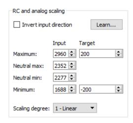
Example Tic scaling settings for RC position control mode.
