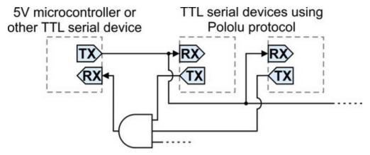
Daisy-chaining multiple TTL serial devices that support the Pololu protocol for control by a single microcontroller.
