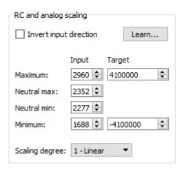
Example Tic scaling settings for RC speed control mode.
