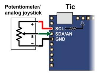
If you are using something other than a potentiometer to generate the analog signal, make sure that the ground node of that device is connected to a GND pin on the Tic, and that the analog signal from that device is connected to the Tic's SDA/AN line. The Tic's analog input can only accept signals between 0 V and 5 V with respect to GND; signals outside of this range could damage the Tic.
