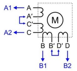
Connecting a two-phase unipolar/ bipolar stepper motor with eight (8) leads to the Tic with the phase coils in series.
