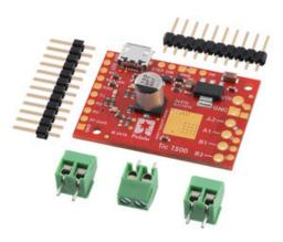
Tic T500 USB Multi-Interface Stepper Motor Controller (without connectors soldered) with included headers and terminal blocks.
