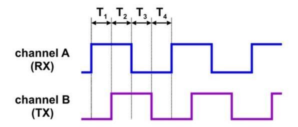
The time between the channel transitions (labeled  $T_{1-4}$  in the diagram above) must be at least 100  $\mu$ s. The signal must rise to 4 V or higher, and must stay within 0 V to 5 V.
