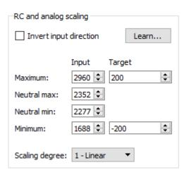
Example Tic scaling settings for RC position control mode.
