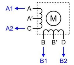
Connecting a two-phase bipolar stepper motor with four (4) leads to the Tic.
