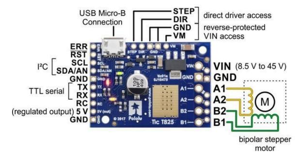
The **Tic T825**, shown above, is based on the DRV8825 IC from Texas Instruments. This driver IC supports microstepping with up to 32 microsteps per full step and features three configurable decay
