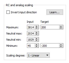
Example Tic scaling settings for analog position control mode.
