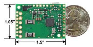
Tic 36v4 USB Multi-Interface High-Power Stepper Motor Controller, bottom view with dimensions.
