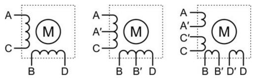
The Tic works with two-phase stepper motors that can be controlled in a bipolar configuration.
