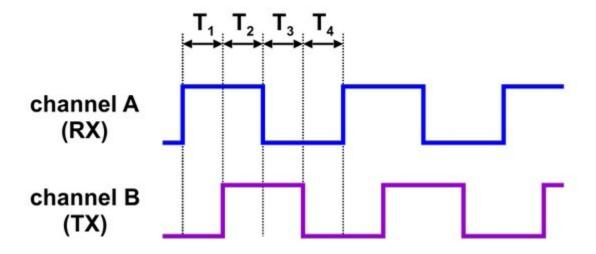
The time between the channel transitions (labeled T<sub>1-4</sub> in the diagram above) must be at least 100 µs.
