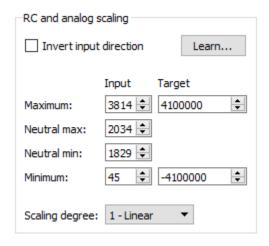
Example Tic scaling settings for analog speed control mode.
