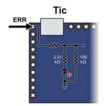
Schematic diagram of the Tic ERR pin when it is acting as an output (i.e. there are errors).
