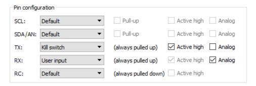
**Example pin configuration settings for a Tic Stepper Motor Controller.**
