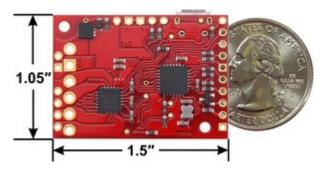
Tic T500 USB Multi-Interface Stepper Motor Controller, bottom view with dimensions. This picture shows the original tic03a version that shipped prior to 3 January 2019.
