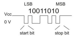
Diagram of a non-inverted TTL serial byte.
