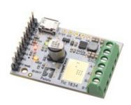
Tic T834 USB Multi-Interface Stepper Motor Controller (Connectors Soldered).
