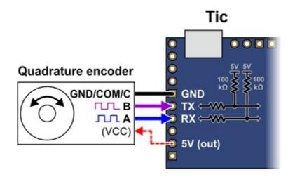
The Tic expects to see a quadrature encoder signal like this on the RX and TX pins:
