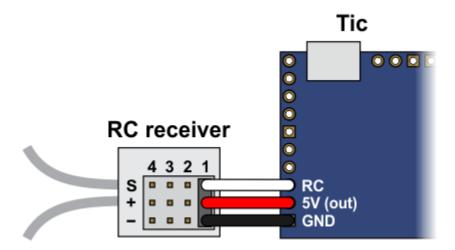
In this configuration, the RC receiver will be powered by the Tic's 5 V regulator via the 5V output pin. If you want to power the receiver from another power source instead, you should **not** connect the Tic's 5V pin to it as doing so would short the two sources together and could damage the Tic or receiver.
