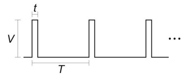
The signal should be low (0 V) normally and have periodic pulses with an amplitude (V) of at least 2 V. The width of the pulses (t) should be between 200  $\mu$ s and 2700  $\mu$ s. The period of the signal (T), should be at most 100 ms, and the there is no particular lower limit. When the Tic has received three good pulses in a row, it writes the width of the latest pulse to the "RC pulse width" variable in units of  $1/12 \mu$ s.
