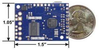
Tic T825 USB Multi-Interface Stepper Motor Controller, bottom view with dimensions.
