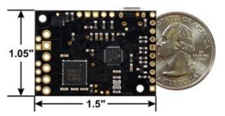
Tic T249 USB Multi-Interface Stepper Motor Controller, bottom view with dimensions.
